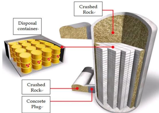
Fig 16. Silo concept diagram.
